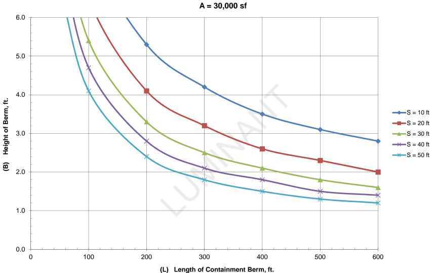
Figure 3. Berm Height vs. Berm Length for Various Setbacks
